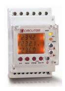
**CVM-MINI** is an instrument that measures, calculates and displays the main electrical parameters in threephase industrial power grids (balanced or unbalanced). The measurement is taken as an RMS value by three AC voltage inputs and three AC current inputs. (through current transformers,  $l_n$ /5A or  $l_n$ /1A/ 250 mA). The measured and calculated parameters are shown in the table of variables.
