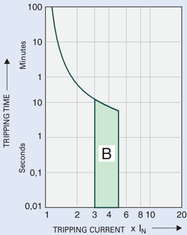
Tripping characteristic B
